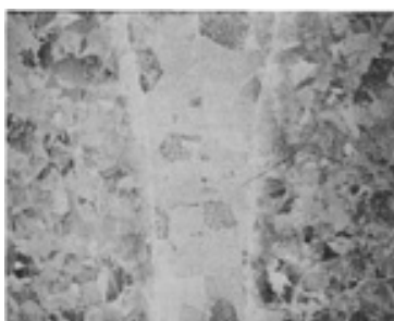
FIG. 6 MACROGRAPH SHOWING COARSE PRIOR-BETA GRAIN SIZE IN AN ELECTRON-BEAM WELDED TI-6AL-4V FORGING. COURTESY OF THE WELDING INSTITUTE
