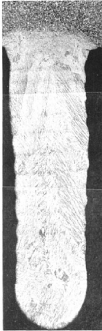
FIG. 23 PHOTOMICROGRAPH OF A TYPICAL AUTOMATIC WIRE-FEED ELECTRON-BEAM REPAIR OF AN AIR SEAL. 15×
