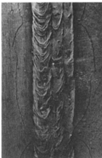
FIG. 2 PWSAC FAILURE IN ALLOY X-750 INDUCED BY RESIDUAL WELDING STRESS AT A 50 MM (2 IN.) THICK JOINT. ALLOY WAS WELDED IN THE AGE-HARDENED CONDITION AND RE-AGED AT 705 °C (1300 °F) FOR 20 H AFTER WELDING.
