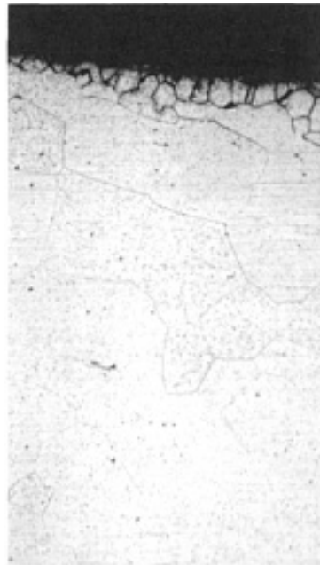
FIG. 14 INTERGRANULAR CORROSION OF THE INSIDE SURFACE HAZ OF E-BRITE STAINLESS STEEL ADJACENT TO THE WELD FUSION LINE. ELECTROLYTICALLY ETCHED WITH 10% OXALIC ACID. 100×. SOURCE: REF 47
