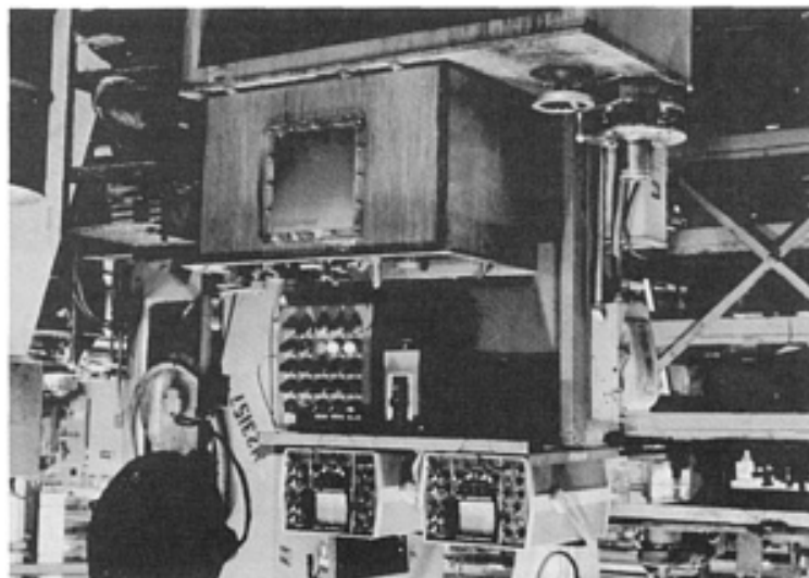
FIG. 10 OVERALL VIEW OF THE ULTRASONIC UNIT USED TO TEST THE ELECTRON-BEAM WELDED ASSEMBLY
