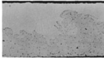
FIG. 6 PHOTOMICROGRAPH SHOWING WELD INTERFACE CROSS SECTION OF 0.08 MM (0.003 IN.) THICK NICKEL ULTRASONICALLY WELDED TO 0.08 MM (0.003 IN.) THICK GOLD-PLATED KOVAR. 300×
