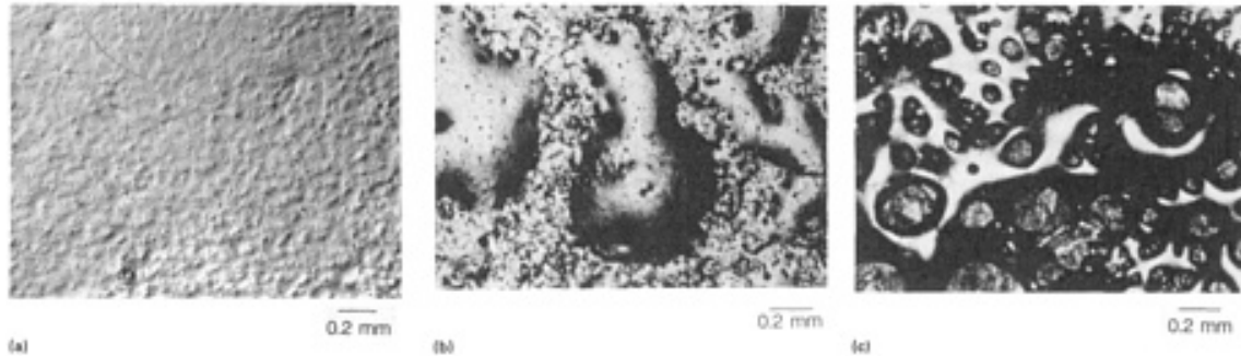
FIG. 18 OPTICAL MICROGRAPHS OF 60SN-40PB SOLDER ON SAMPLE SURFACES. (A) WETTING. (B) DEWETTING. (C) NONWETTING. SOURCE: SANDIA NATIONAL LABORATORIES
