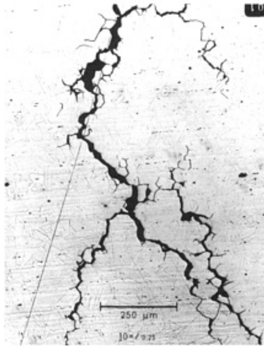
FIG. 13 CAUSTIC SCC IN THE HAZ OF A TYPE 316L STAINLESS STEEL NAOH REACTOR VESSEL. CRACKS ARE BRANCHING AND INTERGRANULAR.
