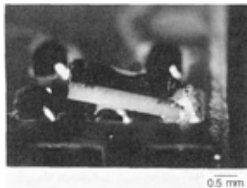
FIG. 12 DRAWBRIDGING OF A LEADLESS CERAMIC CHIP RESISTOR (OPTICAL MACROSCOPY). COURTESY OF SANDIA NATIONAL LABORATORIES
