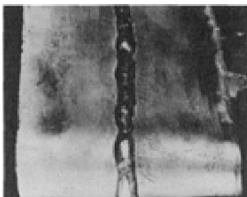
FIG. 4 SULFUR EMBRITTLEMENT OF A JOINT IN ALLOY 200 (UNS N02200). PRIOR TO WELDING, THE CRACKED SIDE OF JOINT WAS WIPED WITH DIRTY CLOTH ON WHICH SULFUR-CONTAINING RESIDUE HAD ACCUMULATED.
