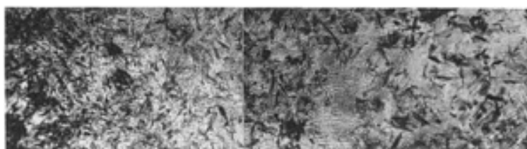
FIG. 2 A TEM MICROSTRUCTURE TRAVERSE ACROSS A MODERATELY COOLED CAPACITOR-DISCHARGE WELD IN AL-8FE-4CE ALLOY. SOURCE: REF 10
