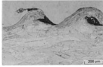
FIG. 6 PHOTOMICROGRAPH SHOWING TYPICAL WAVY WELD INTERFACE OBTAINED WHEN NIOBIUM AND COPPER ARE JOINED BY EXW
