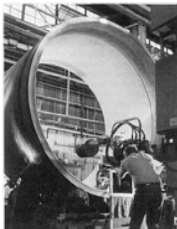
FIG. 36 PLASMA ARC HOT WIRE PROCESS FOR WELD CLADDING THE INTERNAL SURFACE OF A PRESSURE VESSEL SHELL. COURTESY OF NOOTER CORPORATION
