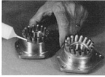
FIG. 12 STAINLESS STEEL TYPE 304 BEVERAGE CAN FILLING NOZZLE. TUBES ARE VACUUM BRAZED WITH A NICKEL BRAZING FILLER METAL AT 1120 °C (2050 °F). LEFT, LOCATION WHERE PASTE ALLOY IS PLACED AROUND TUBE. RIGHT, COMPLETED NOZZLE, SHOWING SMOOTH, VOID-FREE FILLETS. COURTESY OF WALL COLMONOY CORPORATION
