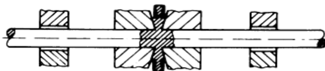
End of second upsetting sequence
