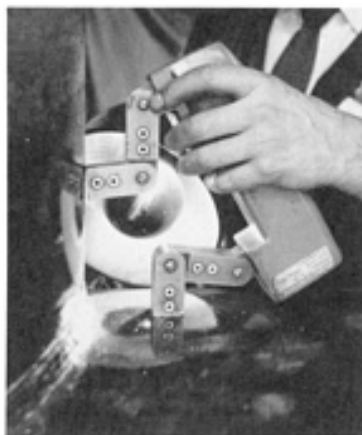
FIG. 2 MAGNETIC-PARTICLE TESTING OF A WELD WITH AN ELECTROMAGNET
