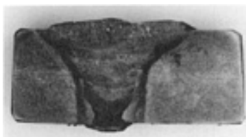
FIG. 8 TRAVERSE SECTION OF THE X-65 PIPE STEEL SHOWN IN FIG. 6 AND 7. PORES IN PASSES 3, 4, 6, AND 9
