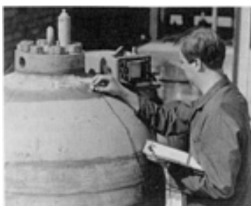
FIG. 5 ULTRASONIC EXAMINATION OF A NOZZLE WELD
