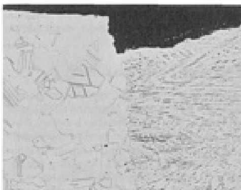
FIG. 2 METALLOGRAPHIC CROSS SECTION SHOWING PREFERENTIAL FUSION ZONE ATTACK IN HASTELLOY B-2 (UNS N10665). SAMPLE WAS A WELDED COUPON PLACED IN A CHEMICAL PLANT PROCESS STREAM FOR APPROXIMATELY 1 YEAR. HYDROCHLORIC AND CHROMIC ACID ETCH. 75×
