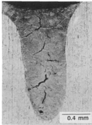
FIG. 10 PULSED ND:YAG LASER-BEAM WELD EXHIBITING SEVERE SOLIDIFICATION CRACKING AS A CONSEQUENCE OF PRIMARY AUSTENITE SOLIDIFICATION, Cr_{eq}/Ni_{eq} = 1.6 . SOURCE: REF 28
