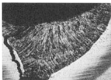
FIG. 7 PHOTOMICROGRAPH OF HYDROGEN-INDUCED CRACK IN HAZ OF WELD. 5×
